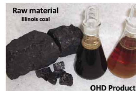
Figure 3. Raw and diluted OHD product derived from Illinois coal.
